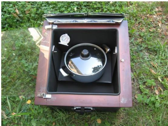
Vessel dimensions should match the dimensions of the inner chamber. In the model PSO-01 the maximum permissible diameter of the pot is 28 cm provided the height is 13.5 cm and the vessel is placed on the sway-tray. The smaller the height the bigger the diameter of the vessel. If the sway-tray is removed, still bigger vessels could be placed.
