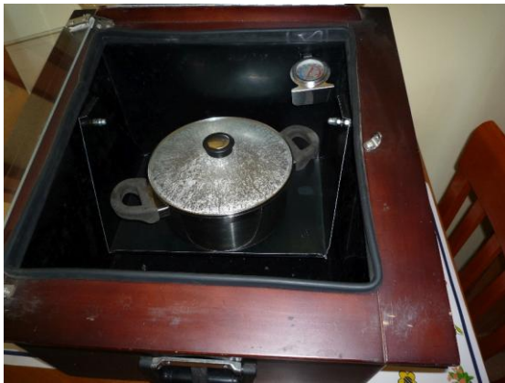
Solar oven PSO-01 used as thermal box or fireless cooker
